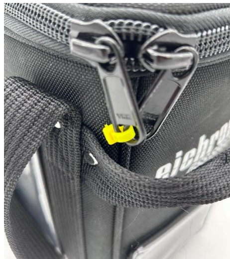
Figure 5: Zip Tie Seal Tightened to Prevent Zipper from opening
