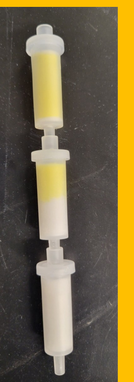
3x 2mL DEHBA cartridges loaded with 100 mg Au. (~35% of capacity)
