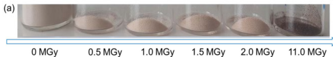
Fig. 3 Pictures of AG MP-50 (a) and SAC (b) before and after exposure to gamma radiation.
