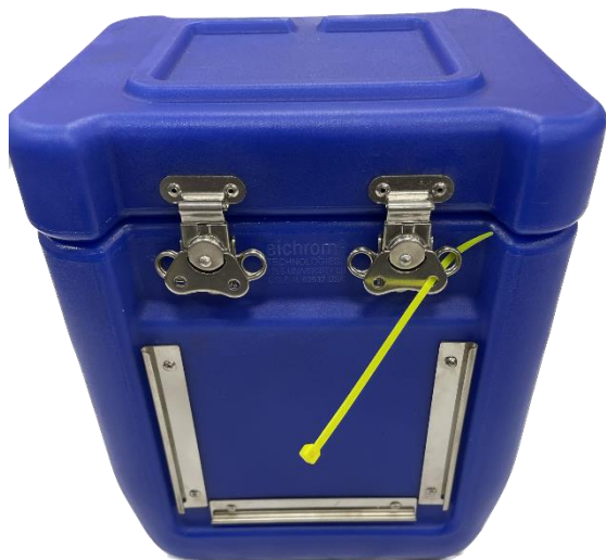
Figure 3: Vial Shield Case - Closed with Latches Locked. Zip Tie Seal Fed Through Spring and Hole in Latch Handle
