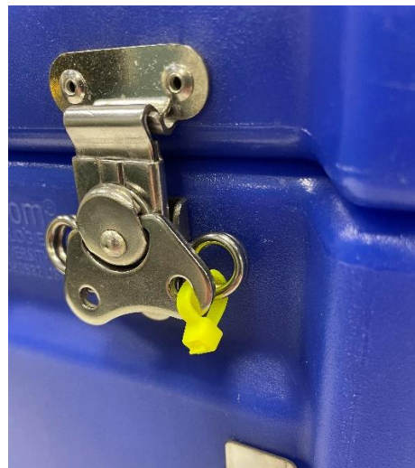
Figure 4: Zip Tie Seal Tightened to Prevent Rotation of the Latch Handle
