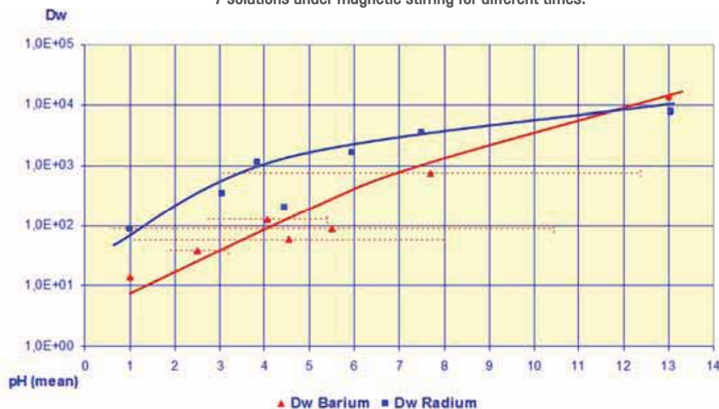
Figure 1: Absorption recovery in Ba-133 on MnO 2 resin. 10mL deionized water, 25 mg of resin, magnetic stirring for 60 minutes at 20°C, pH adjusted with HCl or NaOH. Measurement done with a NaI well-type detector.
