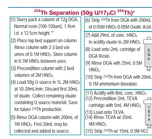
\*Separation is scalable. Simply adjust volumes of the initial DGA column and load solution to accommodate other source sizes.
