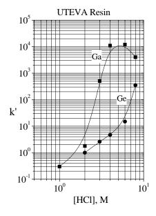
The separation may also be performed using 0.5mL or 1mL columns/ cartridges and proportionally scaled eluate volumes to improve method speed and reduce losses from <sup>68</sup>Ga decay during separation.
