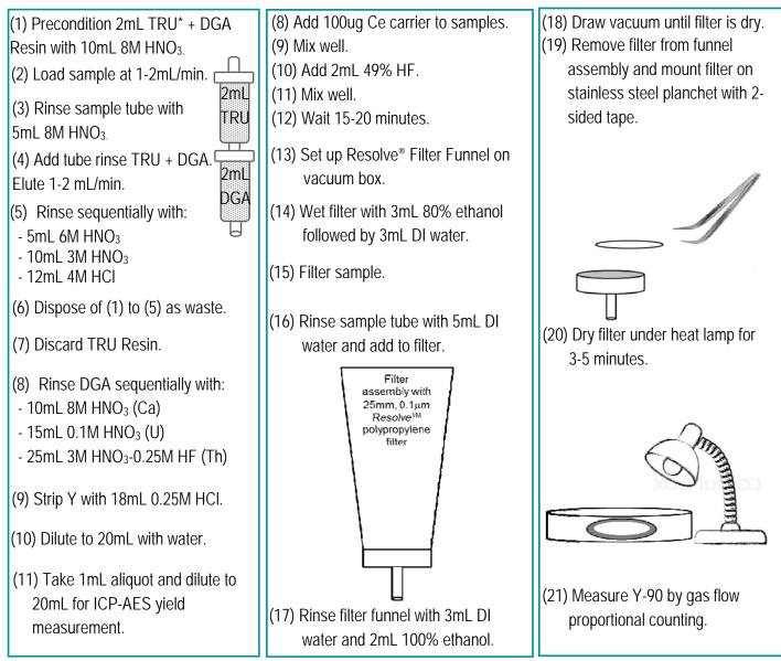
\*TRU Resin improves decontamination factors for U, Th and Bi isotopes, which could interfere with the measurement of <sup>90</sup>Y by gas flow proportional counting.
